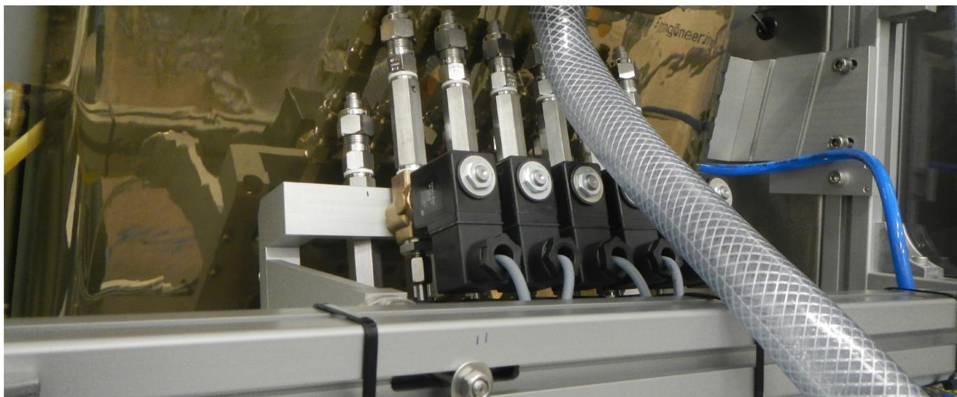
Cleaning system for thin film photovoltaic substrates installed for testing purposes at Flisom's R&D line in Zurich, Switzerland
