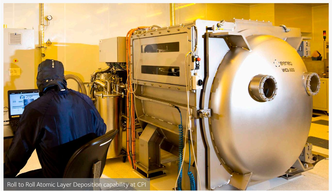
Roll to Roll Atomic Layer Deposition capability at CPI
